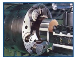
This type of special chucks with hydraulic or pneumatic built-in cylinder has been developed for the threading machining of oil pipes on horizontal lathes.
